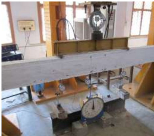
Fig.3 Testing of RC Beam in the laboratory
