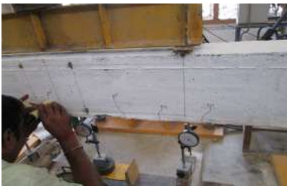
Fig.4 First Crack of RC Beam
