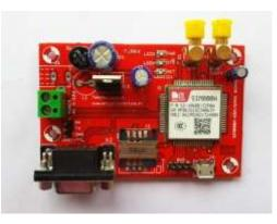
**SIM800A** is a complete Quad-band **GSM**/GPRS solution in a SMT type which can be embedded in the customer **applications**. **SIM800A** support Quad-band 850/900/1800/1900MHz, it can transmit Voice, SMS and data information with low power consumption. It can fit into slim and compact demands of customer design. It will receive data from Arduino microcontroller and act accordingly.
