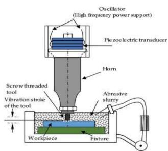
Fig -1: Ultrasonic machining process
