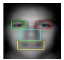
**Fig 3**: The Modular PCA builds multiple eigenfeature in the regions of facial components (e.g., eyes, nose, and mouth) to achieve pose tolerances.
