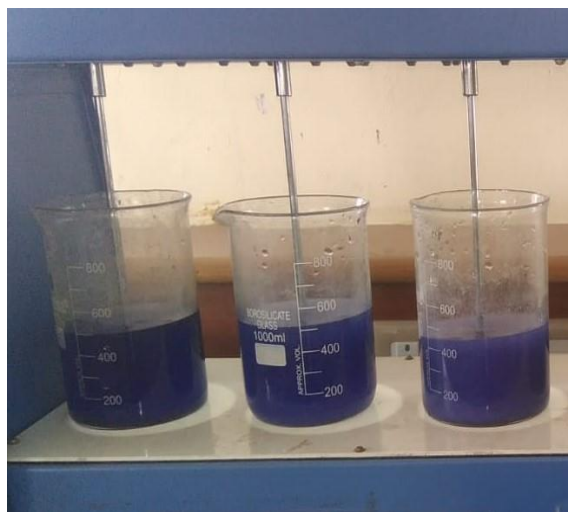
Fig 10: Coagulation by using Jar test apparatus. Fig 11: Filtration of the sample.
