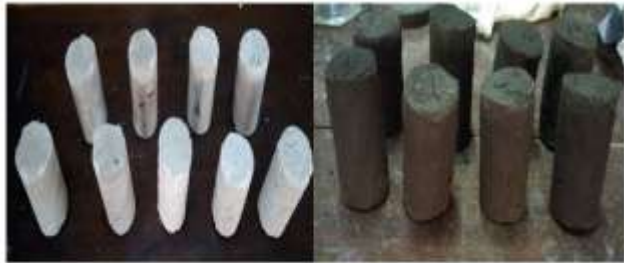
Fig- 1: Fabricated Geopolymers from Kaolin Clay (left) and from Kuttanad Clay (right)
