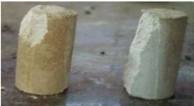
Fig- 3: Cracks induced and failure pattern of the samples caused by efflorescence
