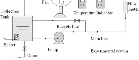
**Project procedure:** This experimental setup includes a reservoir in the form of plastic tank, electrical heater, pump, a flow meter, flow control valves, fan, D.C power supply, temperature sensor, vibrating device and heat exchanger (automobile radiator).
