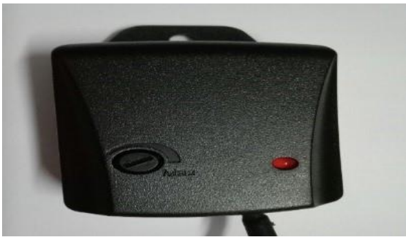
Fig E:Vibration sensor
