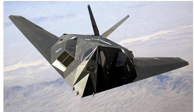
Fig-1. Stealth aircraft it reflects the echo away from radar due to its shape
