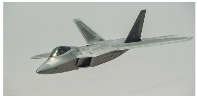
Fig-2. Stealth aircraft it has radiation absorb paint on it so that it absorb the radio wave
