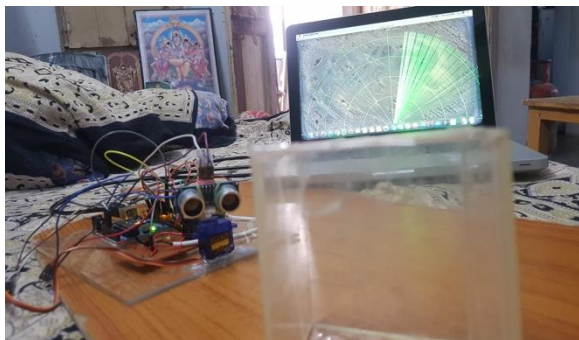
Fig-10. Normal radar with stealth aircraft
