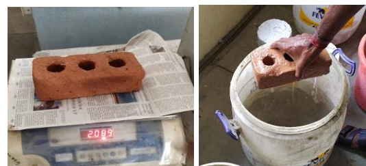
Fig -9: Dry Brick Fig -10: Wet Brick
