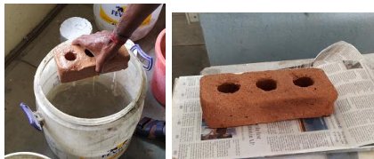
Fig -15: Wet brick Fig -16: Efflorescence Test
