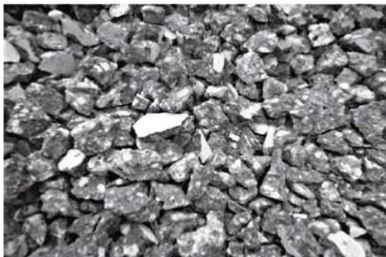
Fig 2 :- Recycled Aggregate By Demolished Construction
