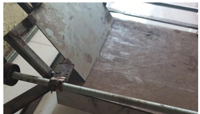
Fig -2.3(a): Ejector movement mechanism
