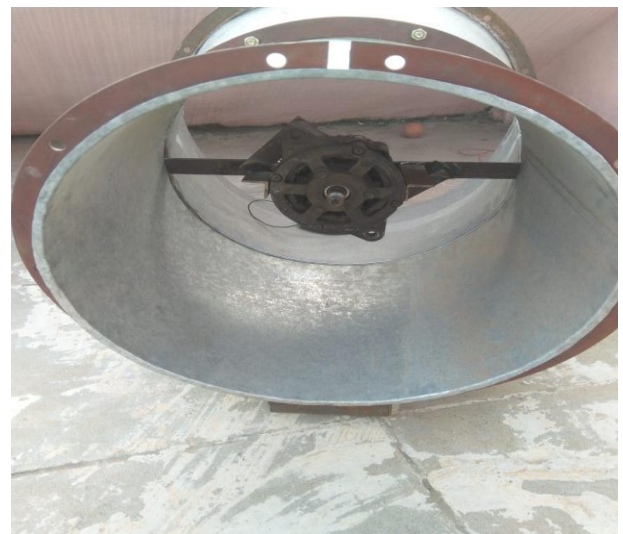
Fig.1- The alternator inside the turbine
