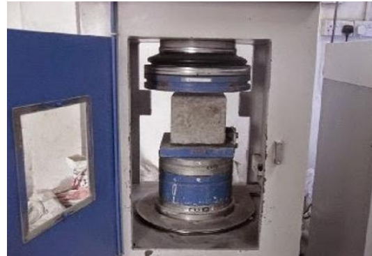
Fig -3: Compressive strength apparatus testing concrete.
