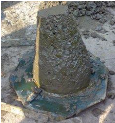
Fig -2: Slump cone test
