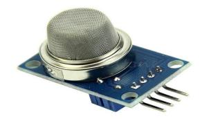
MQ2 measures the smoke, LPG and Corban dioxide. MQ7 measures the Corban monoxide and MQ135 measure the NH3 (ammonia gas) and No.
