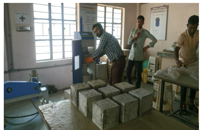
Fig -5: Testing of cube in CTM
