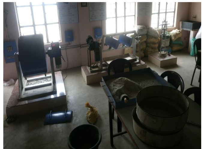
Fig -1: Crushing and grinding of waste glass using Los Angeles Abrasion Testing machine and sieving using 2.36mm size sieve
