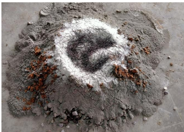
Fig -3: Mixing of cement, sand, aggregate, glass powder and steel fiber.
