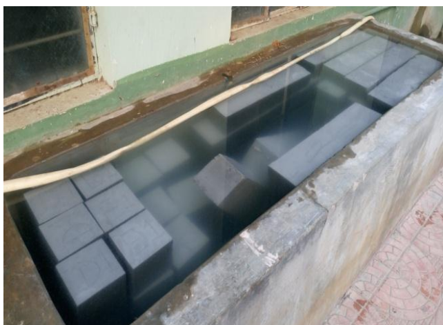
Fig -4: Curing of cubes and beams
