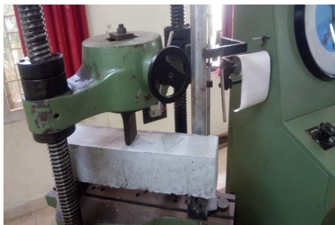
Fig -6: Testing of beam in UTM
