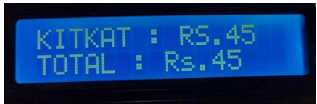
Figure 10 Image displaying the amount of product added to the cart
