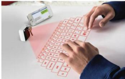
Figure4. Canesta virtual keyboard [1]
