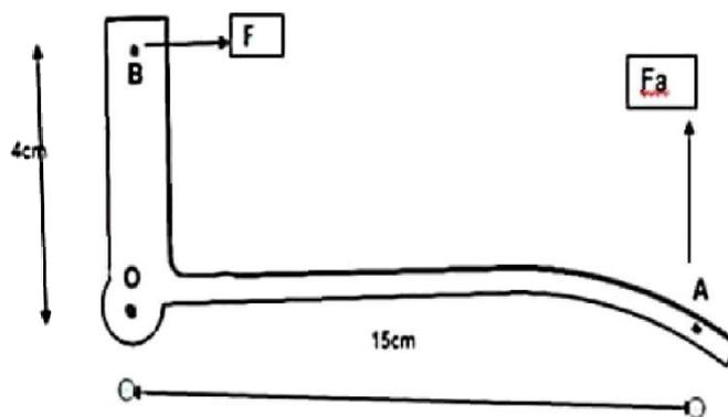
Force ( $F_a$ ) required for holding the work piece is 30N  $F_a = 30\text{ N}$
