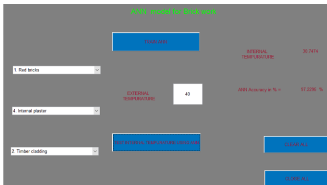
Fig -5: Output generated from the ANN program and the accuracy level and validation internal temperature
