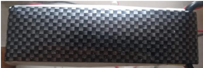
Fig -11: 12v Li-Po Battery 2200mAh
