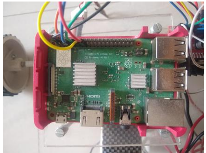
Fig -9: Raspberry Pi 3 Model b+
