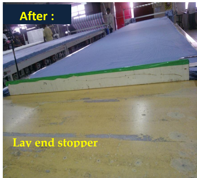
Fig.5.14. Lay end stopper provided
