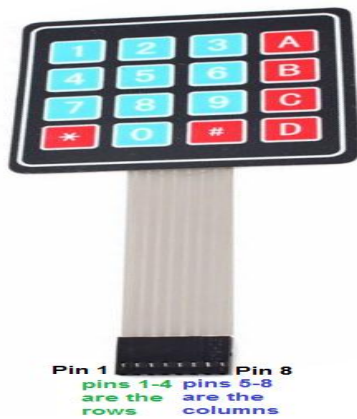
Fig -5: keypad of structure 4*4
