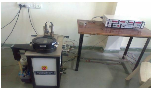
Fig. 3.2 Photograph of experimental set up (Tribometer TR20LE-PHM-400).
