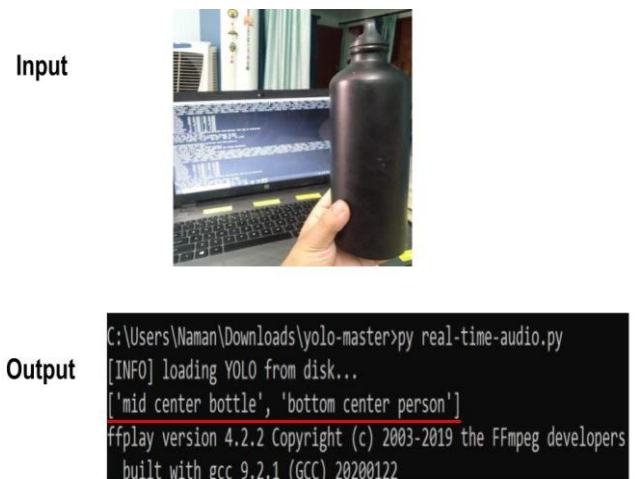
Figure 4: Working of the system which is detecting the bottle and the person holding the bottle.
