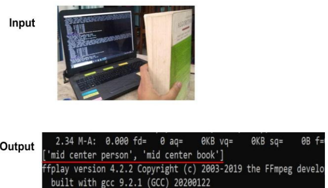
Figure 6: Working of the system which is detecting the book and the person holding the book.
