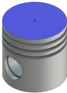
Fig -2: Temperature boundary condition
