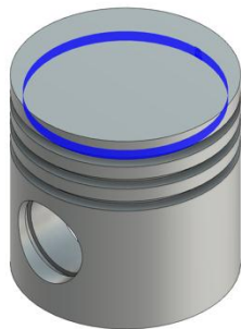
Fig -7: Convection 4 Boundary Condition
