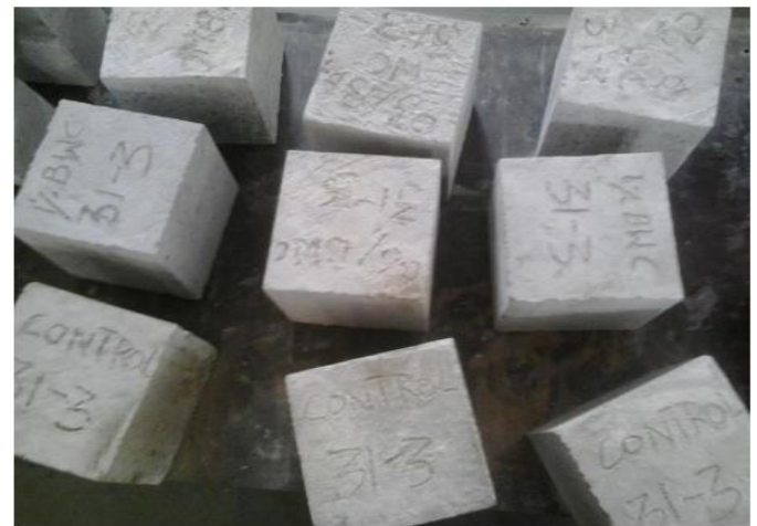
Fig 2 concrete cubes after de-moulding
