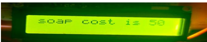
Fig 12: Output from LCD Display when RFID reads the RFID Cards
