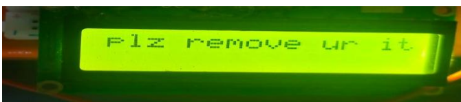
Fig 13: Output from LCD Display when the trolley is full or RFID is not matche\
