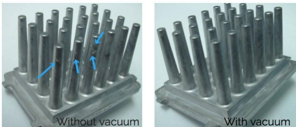
Figure 27: Without vacuum casting (left) With vacuum casting (right)
