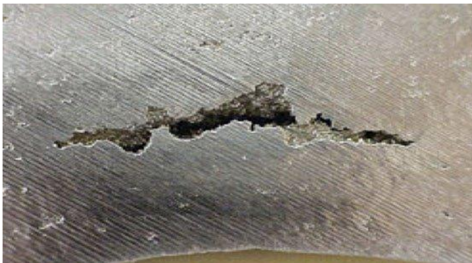
Fig.10: Shrinkage Porosity closed view
