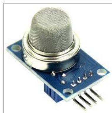
Fig -7: Gas Sensor
