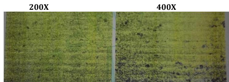
Tool Rotational Speed 900 rpm Welding Speed 20mm/min:
