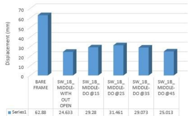
Chart -3: Displacement comparison of one bay SPSW with and without opening
