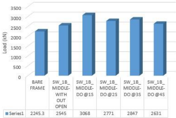
Chart -4: Base shear comparison of one bay SPSW with and without opening
