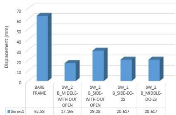
Chart -7: Displacement comparison of two bay SPSW with and without opening
