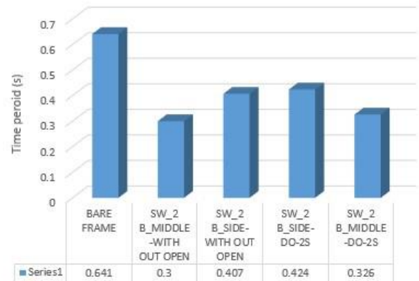
Chart -10: Time period comparison of two bay SPSW with and without opening
