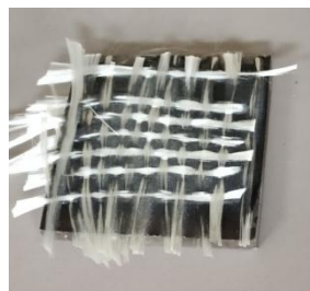
Figure 4: GFRP wrapped With Steel plate
