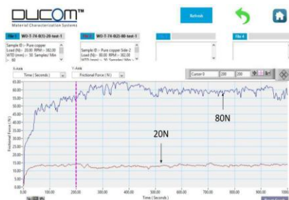
Fig-16: Wear test characteristic graph for pure copper at 20N & 80N load and constant speed
