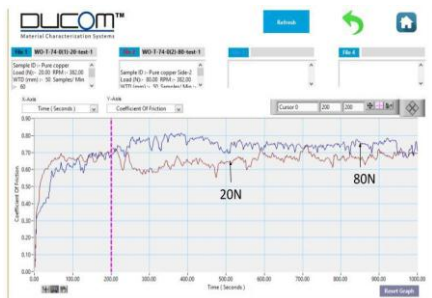
Fig-11: Wear test characteristic graph for pure copper at 20N & 80N load and constant speed
