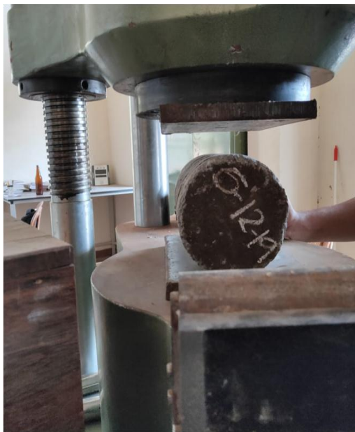
Fig - 5.2: Split Tensile Strength Test set up
