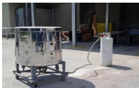
Fig-1: Gas kiln used for fire test
