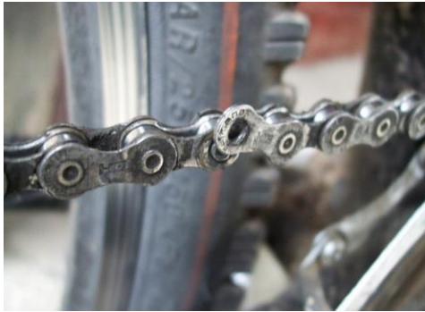
Failure due to repetitive loading (wear and tear).
