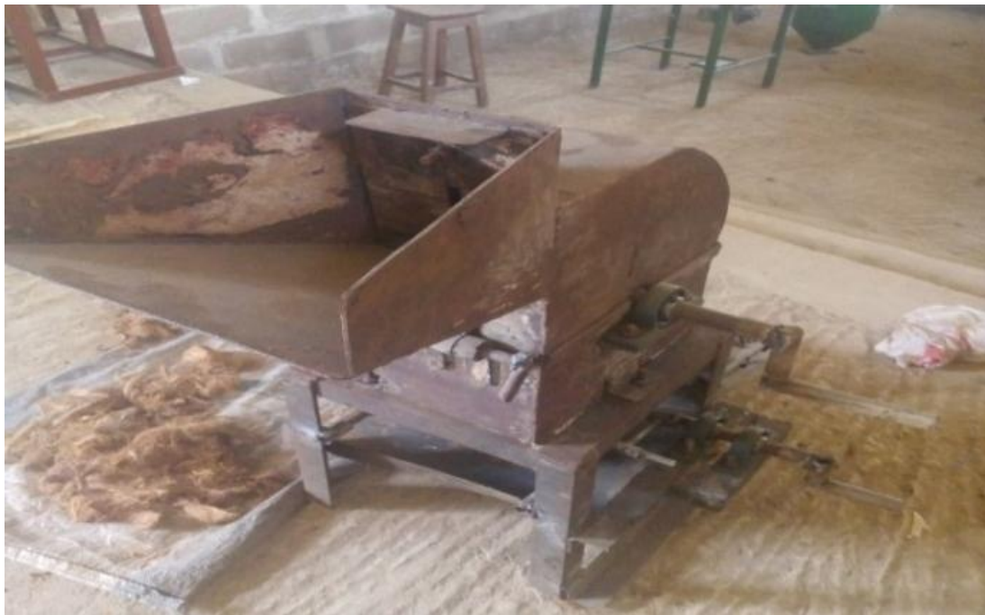
Fig 3: Coir Fibre Extraction and Sieving Machine
