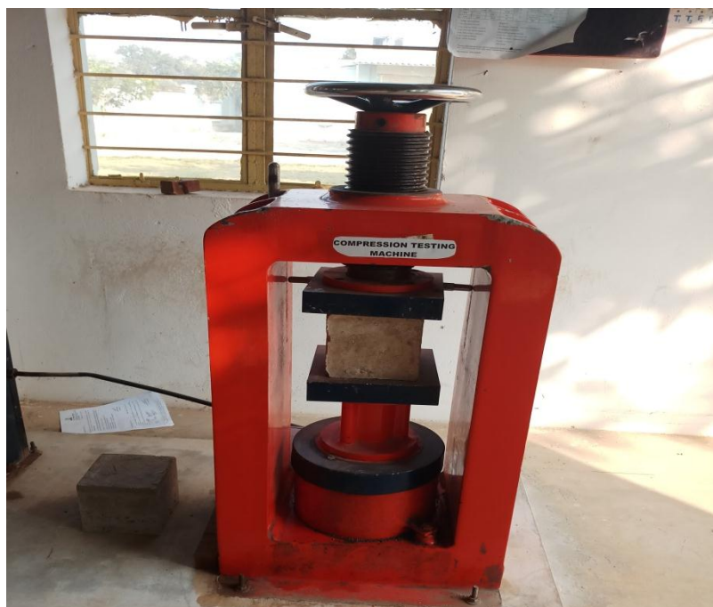
Fig 2- Compressive strength test conducted in lab
