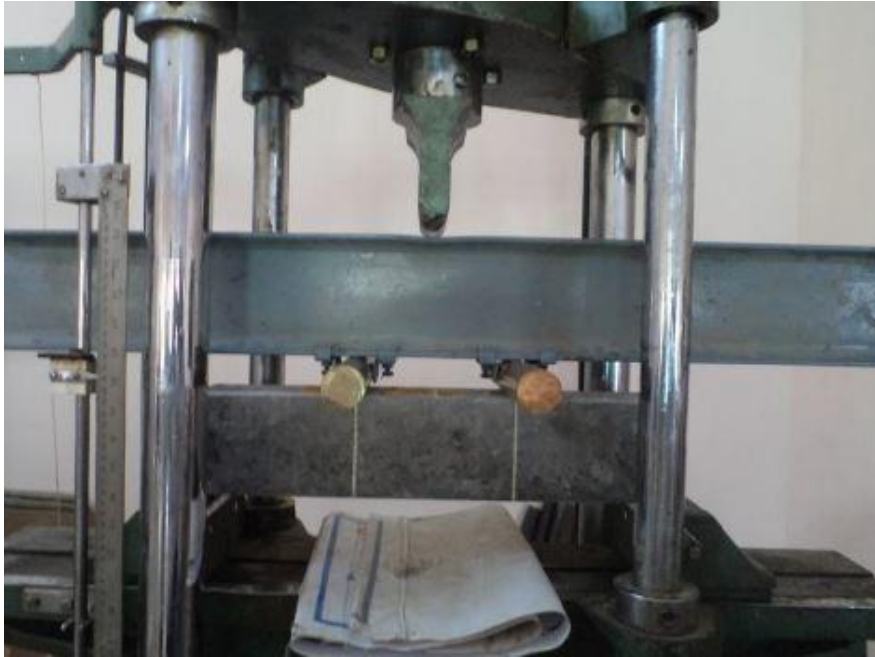
Fig 3- Specimen loading for flexural strength test
