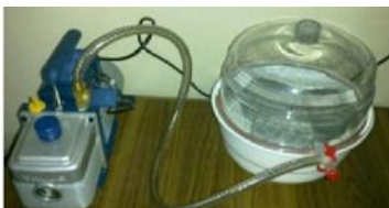
Fig.8 Vacuum pump with desiccator (RCPT)
