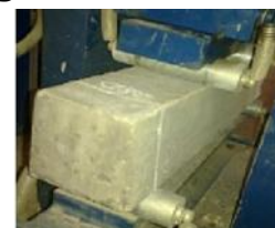
Fig.6 Flexural strength testing on beam
