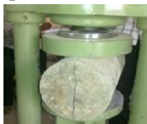
Fig.4 Split Tensile strength test on cylinder
