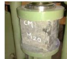
Fig.2 Compressive strength test on cube
