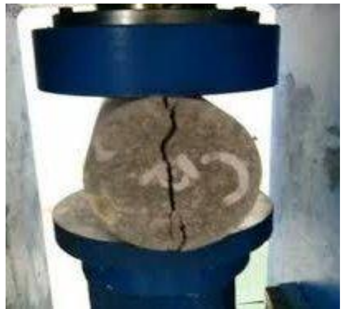
Fig.2 Split tensile testing
