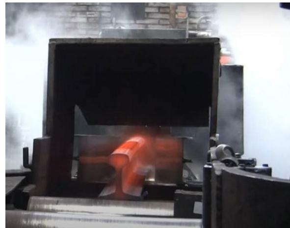
Fig 11: Specimen coming out of SQF after HT
