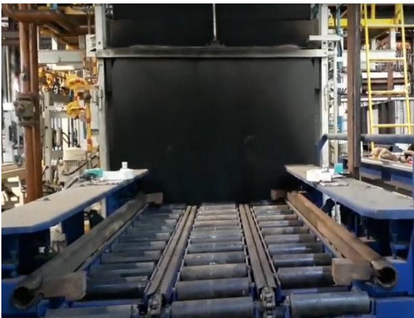
Fig 10: Sealed Quench furnace (SQF)
