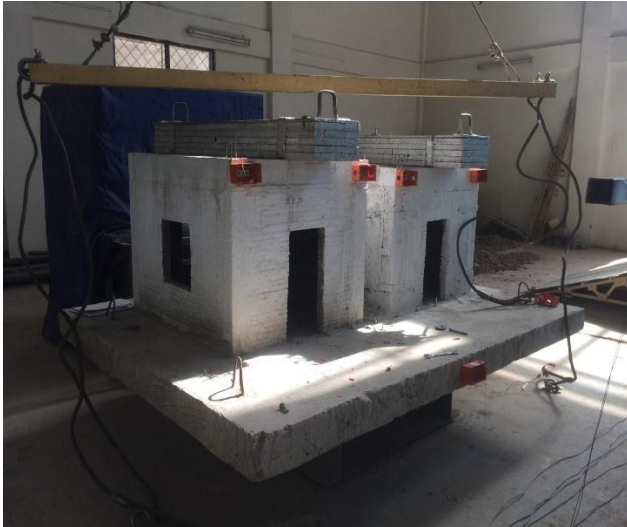
Figure 2: Shake Table mounting of completed model
