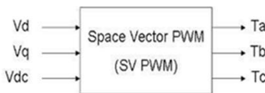
Fig. 5: SVPWM Pulse Generation
