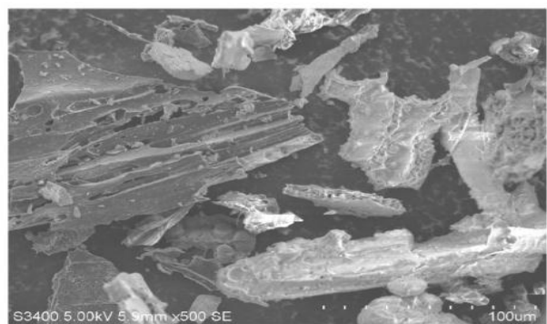
Fig 4: SEM analysis of 90µm fine bagasse ash at 100µm magnification
