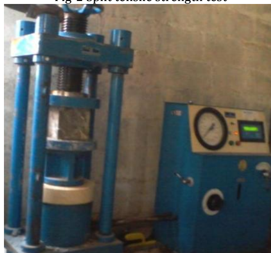
Fig-3 Compressive strength test
