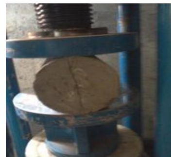
Fig-2 Split tensile strength test
