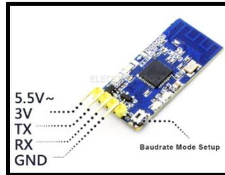
**Fig-11:** Zigbee Module
