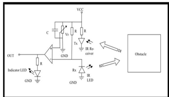
**Fig-9:** Functional Block Diagram of IR Sensor
