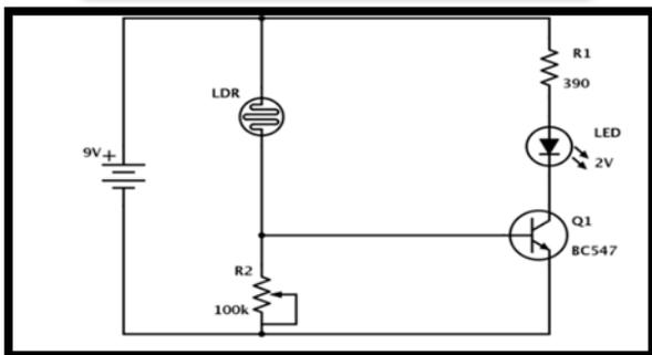
**Fig-10:** Symbolic Representation of LDR Sensor and Circuit diagram of LDR Sensor
