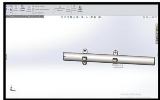
**Fig-5:** Central shaft on which the body of the PI Robot rests
