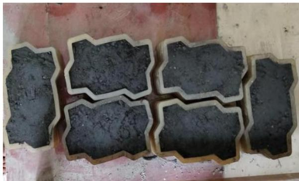
Fig. 5 – Casting of paver blocks with replacement of sugarcane bagasse ash.
