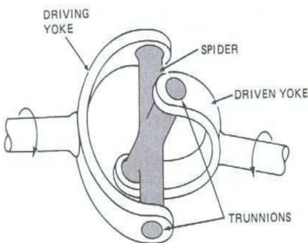
Figure 1.1 universal joints (Cardan joint)
