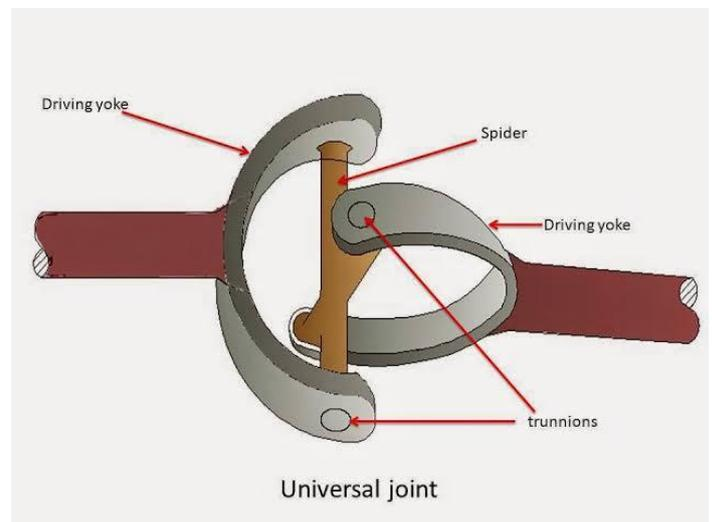
Figure 1.1 Basic structure of universal joint (Cardan joint)
