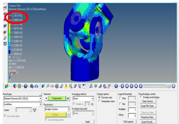
Figure 6.5 Checking stress for modified component
